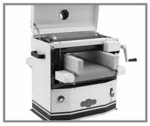
Figure 27. Gauge boards in position.
